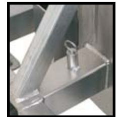
Housing for the transport of the stabilizing legs.
