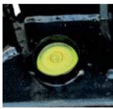
Ground level monitor Vial
