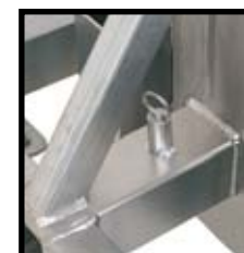
Safety fixation for the stabilizing legs.
