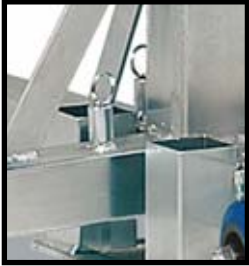
Housing for the transport of the stabilizing legs.
