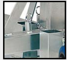
Housing for the transport of the stabilizing legs.
